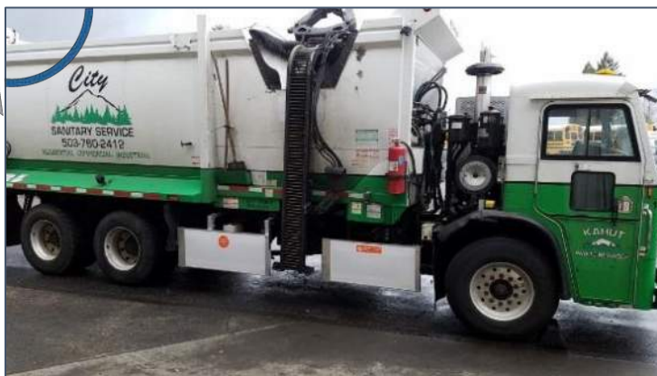
Figure 3-2: Examples of Truck Side Guards
