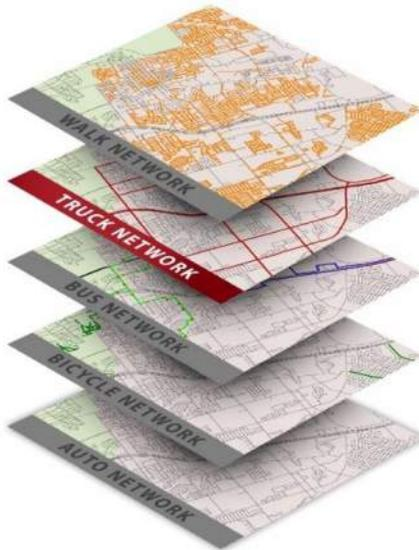
The definition of Functional Classes for the **truck network** is intended to inform the street design process of the needs and impacts of trucks. This Functional Classification system is a tool to define a hierarchy of street facilities as used by trucks.
