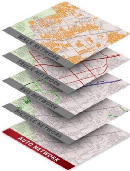
The **auto network** is the base layer for the Thoroughfare Plan, with Functional Classes defined as providing a balance of access and mobility.
