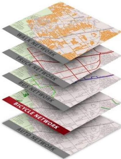
While the basis for a Functional Classification system for the auto network is primarily that of balancing the purposes of access and mobility, in contrast, the basis for the **bicycle network** Functional Classification system can be seen primarily as addressing safety, which in turn directly affects convenience and building ridership volumes. Each of the bicycle Functional Classes therefore has multiple roles in developing a balanced regional multimodal network.
